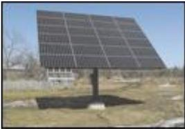
This tracker system, owned by Don Hanson, allows sunlight to be hitting the surface of the solar panel at the optimum position.
